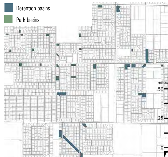
[Figure VII.49] DETENTION BASINS IN PALMDALE, SOME DOUBLING AS PARKS. Source: City of Palmdale]
